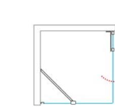
■ Flexible side wall support bar allows you to set different angles and also solves any wall irregularities
