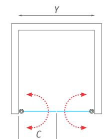
! Nominal sizes of shower enclosures are designed for INSTALLATION ON THE TRAY and they are always assembled with indentation from the edge of the tray. With INSTALLATION ON THE TILES there is a risk, that the size of shower enclosure will be smaller than measured width of the tiles. It is necessary to follow the size charts on "TECHNICAL SPECIFICATION" pages at the end of our catalogue (p. 199–217).
