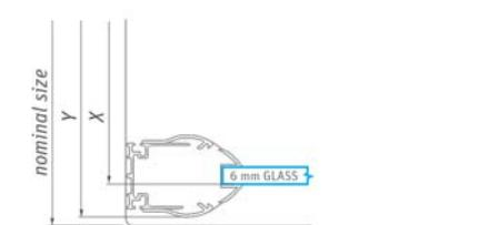
■ Lifting profile with threshold strip and bottom seal
