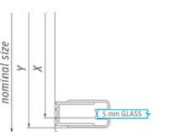
! Nominal sizes of shower enclosures are designed for INSTALLATION ON THE TRAY and they are always assembled with indentation from the edge of the tray. With INSTALLATION ON THE TILES there is a risk, that the size of shower enclosure will be smaller than measured width of the tiles. It is necessary to follow the size charts on "TECHNICAL SPECIFICATION" pages at the end of our catalogue (p. 199–217).
