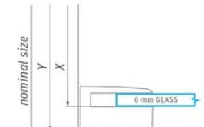
! Nominal sizes of shower enclosures are designed for INSTALLATION ON THE TRAY and they are always assembled with indentation from the edge of the tray. With INSTALLATION ON THE TILES there is a risk, that the size of shower enclosure will be smaller than measured width of the tiles. It is necessary to follow the size charts on "TECHNICAL SPECIFICATION" pages at the end of our catalogue (p. 199–217).
