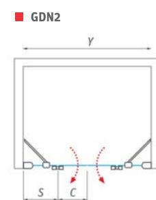
\* GDN2 as an atypical up to 2 000 mm only for installation to a niche. In combination with a fixed panel UB only up to 1 500 mm.
