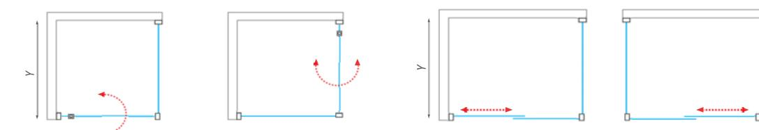
! Nominal sizes of shower enclosures are designed for INSTALLATION ON THE TRAY and they are always assembled with indentation from the edge of the tray. With INSTALLATION ON THE TILES there is a risk, that the size of shower enclosure will be smaller than measured width of the tiles. It is necessary to follow the size charts on "TECHNICAL SPECIFICATION" pages at the end of our catalogue (p. 199-217).
