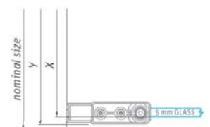
Nominal sizes of shower enclosures are designed for INSTALLATION ON THE TRAY and they are always assembled with indentation from the edge of the tray. With INSTALLATION ON THE TILES there is a risk, that the size of shower enclosure will be smaller than measured width of the tiles. It is necessary to follow the size charts on "TECHNICAL SPECIFICATION" pages at the end of our catalogue (p. 199–217).
