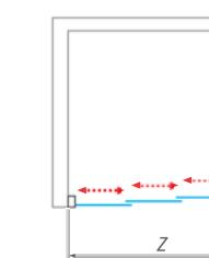
Nominal sizes of shower enclosures are designed for INSTALLATION ON THE TRAY and they are always assembled with indentation from the edge of the tray. With INSTALLATION ON THE TILES there is a risk, that the size of shower enclosure will be smaller than measured width of the tiles. It is necessary to follow the size charts on "TECHNICAL SPECIFICATION" pages at the end of our catalogue (p. 199-217).
