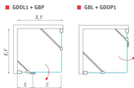
! Nominal sizes of shower enclosures are designed for INSTALLATION ON THE TRAY and they are always assembled with indentation from the edge of the tray. With INSTALLATION ON THE TILES there is a risk, that the size of shower enclosure will be smaller than measured width of the tiles. It is necessary to follow the size charts on "TECHNICAL SPECIFICATION" pages at the end of our catalogue (p. 199-217).
